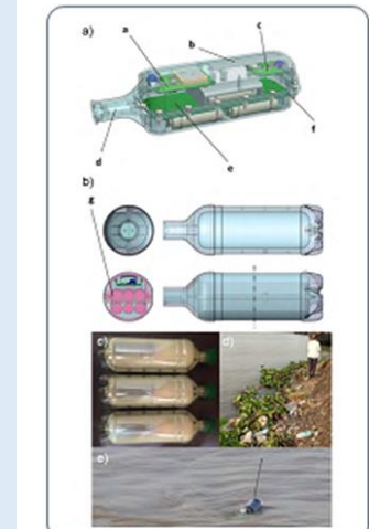
Figure 1. The shape and profile of the bottle tag: a) Transparent schematic showing the seating of batteries and placement of electronics inside the bottle's enclosure; a = Horizon GPS board, b = Cellular antenna, c = Cellular or Ar-gos satellite board, d = CNC-milled enclosure, e = Battery board, f = O-ring seal. b) Transparent top, side, bottom view and orientation of batteries inside the bottle's internal cavity; g = Positioning of AA lithium batteries c) Phase A GSM bottle tags d) Observed PET bottles in river bank Ganges River e) Phase II satellite bottle tag after deployment. (Photos (c) and (d) by Emily Duncan Photo (e) by Alasdair Davies)
